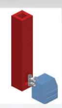
Place inspection unit and connection tee in the cut opening.
