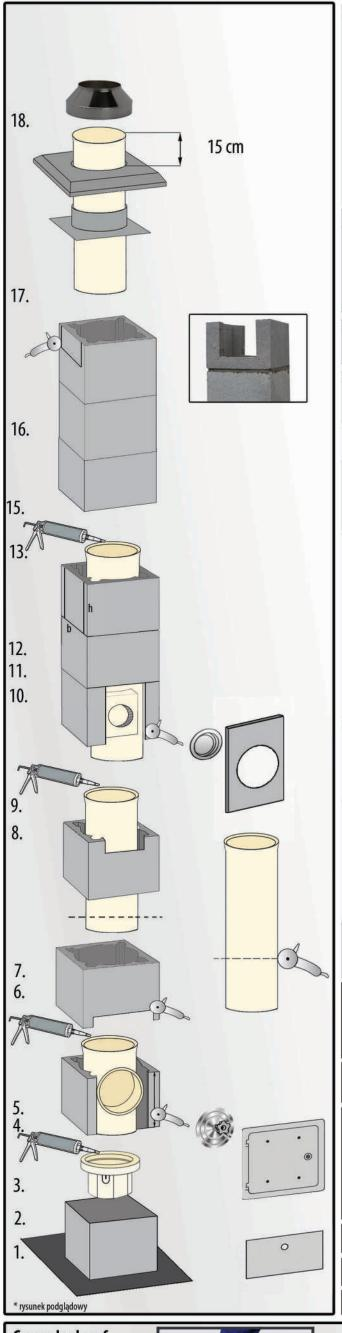
17. Cut the last pipe, so that it outstands 15cm over the cover plate (the bell part should be cut off). Mount the pipe. Seal the joint between the cover plate and the formwork, using roofing silicone. Mount the end cone stabilizer 7cm below the top of the last pipe. Tighten the adjustment on the stabilizer. Put silicone on the top of the pipe. Mount the end cone, until you hear a click.
