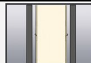
Correctly joined pipes without excess silicone inside.
