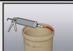
Put the right amount of silicone into the pipe bell.
